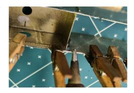
7. The rivet overlays (9, 10, 11, 12 and 13) for both the ends and along the top of the beam are attached using the same method. Be sure that they are level with the top edge and that a small off cut of the etched fret can pass down into the slots.
