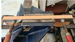
NOTE: It is imperative that both ends of the bridge are straight and square to the central mounting block. This ensures that the track will align when a through track is modelled and the bridge is turned 180 degrees. I have included a special 10mm acrylic jig so the bridge beam can be clamped straight and square.
