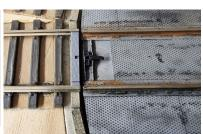
**35.** I have not included rail for the bridge with the kit as modellers tend to use varying sizes for their layouts. Its been designed for use with Code 70 rail however other sizes can be used. Cut two lengths of rail the length of the bridge and glue these down between the details of the urethane strips. I used Pliobond for this but thick Superglue (green zap-a-gap) could also be used.
