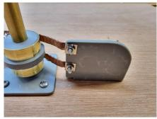
17. Fit the two springs to the ends of the braid then onto the other bracket. You may need to open out the ends of the springs and adjust their length to achieve light spring tension on the braid. I found this method to be very reliable especially when sound equipped locomotives are being turned with their sound and light functions active.
