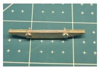
12. Using a steel ruler or similar, fold the protruding areas to 90°.
