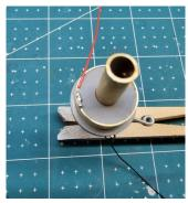
6. Trim the wires so they protrude about 15mm out from the top of the shaft. Fit the included heat shrink tube to the wires and solder the two wires to the female two pin connector. This connector needs to fit neatly into the slot in the top of the 3D printed deck block (see step 11). It may require some light sanding or filing to make it fit.
